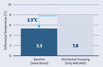
The design Delta T is 7 °C. Before the distributed pumping concept, its Delta T was 5.3 °C, which increased to 7.8 °C after introducing the concept.
